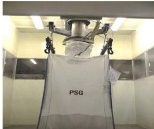
Figure 5: Big-Bag Filling Head
