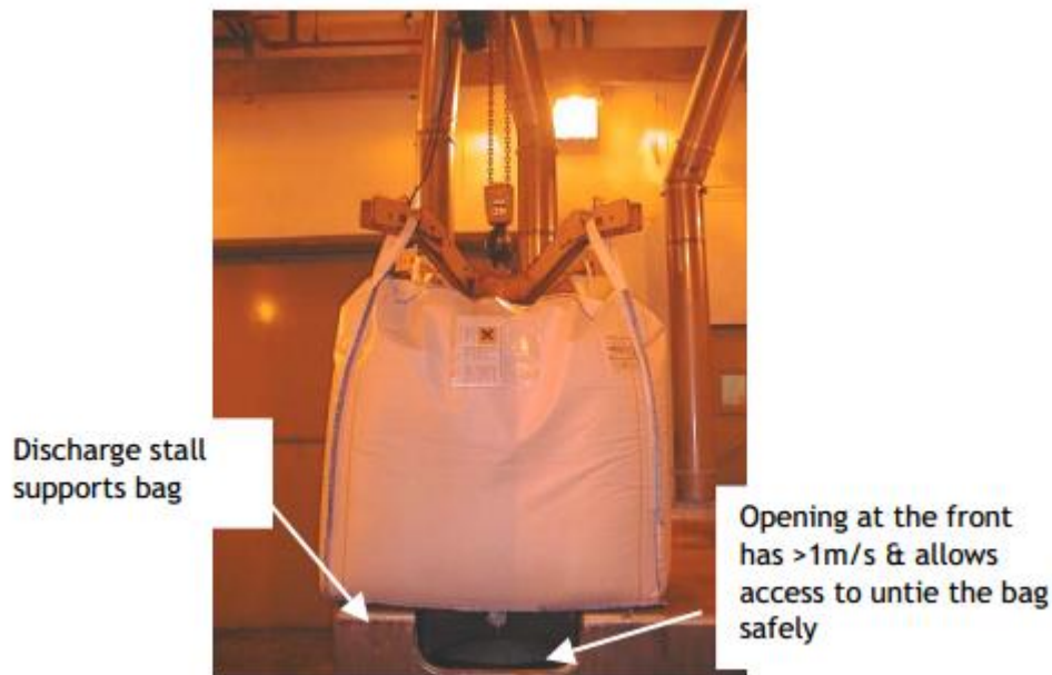
Figure 2 : Enzyme Bag Discharge
